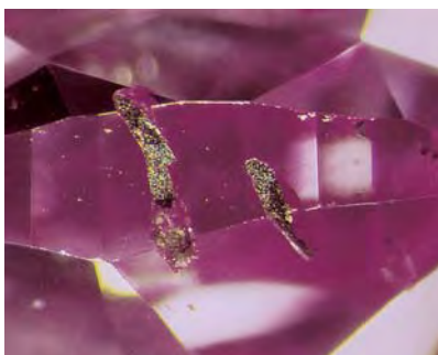
Figure 9. This photomicrograph shows the residue-filled surface cavities along the girdle of the diamond. Chemical analysis by EDXRF revealed the presence of Fe and Ca in the residue. Magnified 60×.
