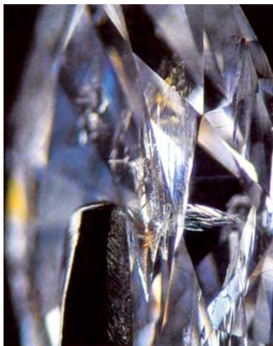
Figure 13. In profile, the stone in figure 12 can be seen to contain naturally iridescent unfilled fractures (to the right of the tweezer) as well as a blue flash effect (visible throughout the region to the left) from reflections of filled fractures. Magnified 20×.
