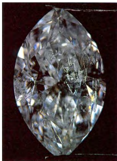
Figure 12. Some of the fractures in this 1.48 ct marquise are filled and others are unfilled.
