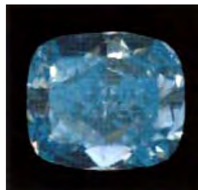
Figure 3. As shown here for the 5.69 ct stone, the type IIb blue diamonds displayed very strong blue phosphorescence to short-wave UV that lasted more than 60 seconds.
