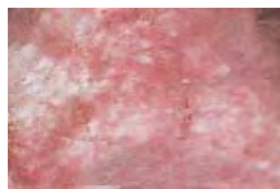
Figure 10. At 10× magnification, the roiled appearance of the coloration in the unusual mottled quartzes shown in figure 9 could be seen.
