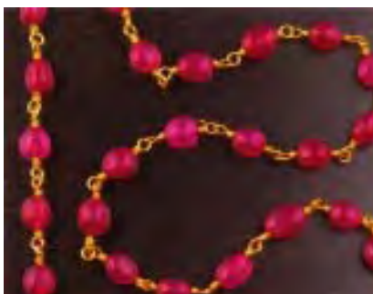
Figure 11. The 29 beads in this necklace are quartzite that has been dyed to imitate ruby (left). The dye fluoresces orange to long-wave UV radiation (right). The fluorescing dye can sometimes be seen defining the grain boundaries and/or other surface-reaching fractures it fills.
