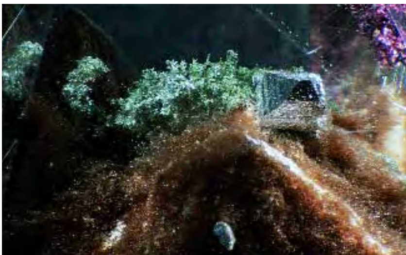
Figure 8. Raman analysis of similar inclusions revealed that the 1-cm-long “lizard’s” body and tail are composed of chlorite, while its head is an anatase crystal.
