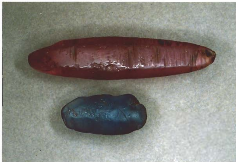
Figure 10. These two apparently waterworn corundum crystals, 56.04 and 21.80 ct, are actually flame-fusion synthetic sapphires. Photo courtesy of the Swiss Foundation for the Research of Gemstones (SSEF).
