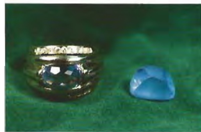
Figure 16. Both of these synthetic spinels were originally sold as topaz. The stone set in the ring measures 11.0 × 6.8 × 7.5 mm; the loose preform measures 15.0 × 10.0 × 10.0 mm.
