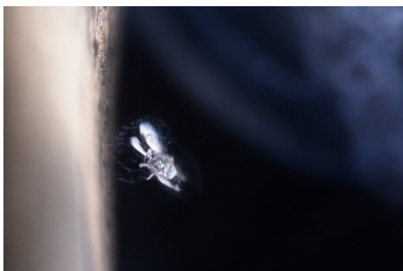
Figure 22: Sample 6543 (Cambodia), heated at 1050°C for 28 hours, partially healed fracture developed on an unidentified colorless crystal , darkfield illumination, FOV 1.05 mm, photomicrographs by C. Khowpong © GIA.
