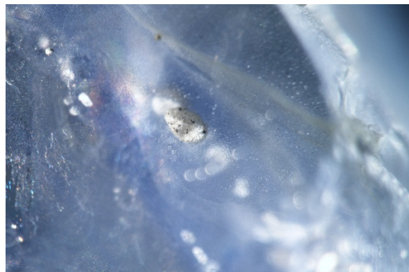
Figure 61: Sample 9300 (Thailand), heated at 1500°C for 7 hours, the yellow stain was removed and crystal altered to a frosty white form , fiber-optic illumination, FOV 1.75 mm, photomicrographs by C. Khowpong © GIA.
