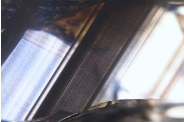
Figure 56: Sample 9300 (Thailand), heated at 1500°C for 7 hours, internal diffusion , diffused light illumination, FOV 4.80 mm, photomicrographs by C. Khowpong © GIA.
