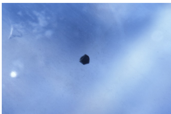
Figure 66: Sample 9129 (Thailand), heated at 1500°C for 7 hours, the angular ferrocolumbite changed to round shape and dot-like fingerprint developed around the crystal , darkfield and fiber-optic illumination, FOV 1.75 mm, photomicrographs by C. Khowpong © GIA.
