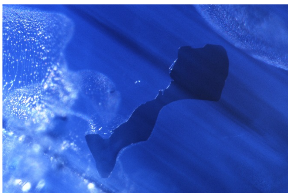
Figure 25: Sample 4246 (Australia), heated at 1050°C for 28 hours, no signs of alteration to molybdenite platelet , darkfield illumination, FOV 1.05 mm, photomicrographs by C. Khowpong © GIA.
