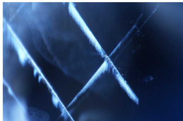
Figure 58: Sample 2390 (Cambodia), heated at 1500°C for 7 hours, no signs of alteration to growth tubes , fiber-optic illumination, FOV 1.40 mm, photomicrographs by C. Khowpong © GIA.
