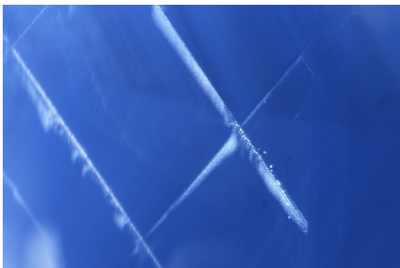
Figure 58: Sample 2390 (Cambodia), heated at 1500°C for 7 hours, no signs of alteration to growth tubes , fiber-optic illumination, FOV 1.40 mm, photomicrographs by C. Khowpong © GIA.
