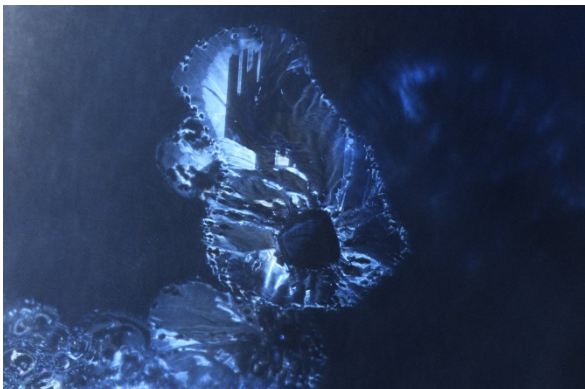
Figure 73: Sample 0881(Australia), heated at 1500°C for 7 hours, thin film around feldspar crystal altered to discoid fracture , fiber-optic illumination, FOV 1.75 mm, photomicrographs by C. Khowpong © GIA.
