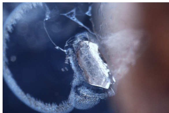
Figure 24: Sample 7132 (Cambodia), heated at 1050°C for 28 hours, no alteration to zircon crystal but partially healed fracture developed around the crystal , darkfield illumination, FOV 1.20 mm, photomicrographs by C. Khowpong © GIA.
