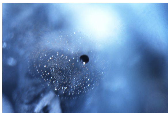
Figure 66: Sample 9129 (Thailand), heated at 1500°C for 7 hours, the angular ferrocolumbite changed to round shape and dot-like fingerprint developed around the crystal , darkfield and fiber-optic illumination, FOV 1.75 mm, photomicrographs by C. Khowpong © GIA.
