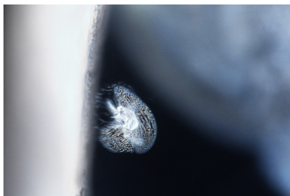
Figure 22: Sample 6543 (Cambodia), heated at 1050°C for 28 hours, partially healed fracture developed on an unidentified colorless crystal , darkfield illumination, FOV 1.05 mm, photomicrographs by C. Khowpong © GIA.
