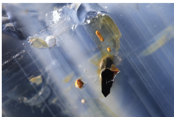
Figure 60: Sample 9300 (Thailand), heated at 1500°C for 7 hours, yellow stain along fractures was removed, the black crystal disappeared and fractures changed to dot-like partially healed fractures , fiber-optic illumination, FOV 1.75 mm, photomicrographs by C. Khowpong © GIA.
