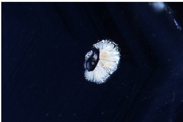
Figure 78: Sample 7159 (Cambodia), heated at 1500°C for 7 hours, thin film around feldspar crystal developed partially healed fracture at rim , fiber-optic illumination, FOV 1.05 mm, photomicrographs by C. Khowpong © GIA.
