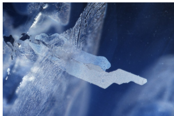
Figure 27: Sample 4246 (Australia), heated at 1050°C for 28 hours, transparent fluid inclusion altered to an opaque frosty white form , darkfield illumination, FOV 1.40 mm, photomicrographs by C. Khowpong © GIA.
