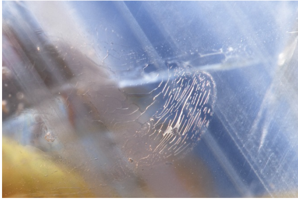
Figure 62: Sample 9300 (Thailand), heated at 1500°C for 7 hours, minor alteration to a fluid fingerprint and minute particles dissolved , fiber-optic illumination, FOV 1.75 mm, photomicrographs by C. Khowpong © GIA.
