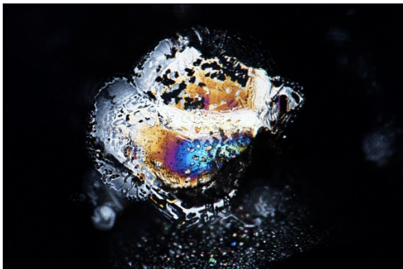
Figure 79: Sample 7159 (Cambodia), heated at 1500°C for 7 hours, alteration to iridescence thin film at rim , fiber-optic illumination, FOV 1.05 mm, photomicrographs by C. Khowpong © GIA.
