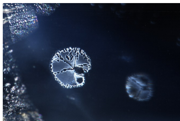
Figure 29: Sample 9424 (Australia), heated at 1050°C for 28 hours, no signs of alteration to feldspar crystal and thin film , fiber-optic illumination, FOV 1.05 mm, photomicrographs by C. Khowpong © GIA.
