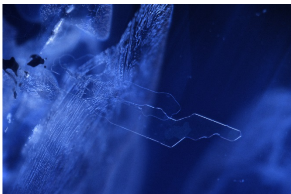
Figure 27: Sample 4246 (Australia), heated at 1050°C for 28 hours, transparent fluid inclusion altered to an opaque frosty white form , darkfield illumination, FOV 1.40 mm, photomicrographs by C. Khowpong © GIA.
