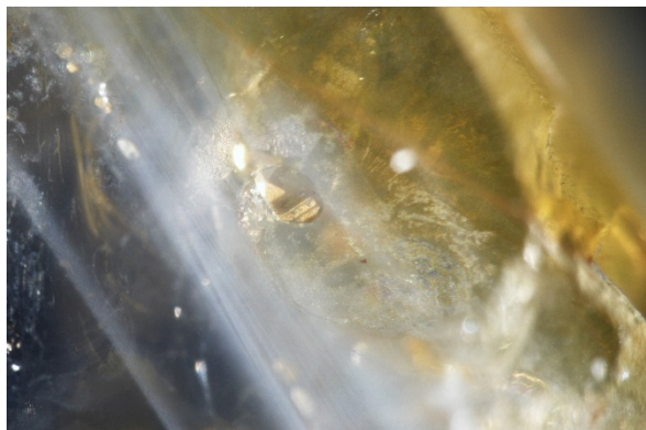
Figure 61: Sample 9300 (Thailand), heated at 1500°C for 7 hours, the yellow stain was removed and crystal altered to a frosty white form , fiber-optic illumination, FOV 1.75 mm, photomicrographs by C. Khowpong © GIA.
