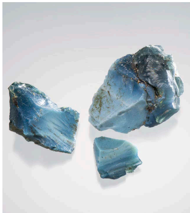
Figure 45. Rough “Swedish Blue” slag byproduct. Photo by Kevin Schumacher; courtesy of Atle Berger.
