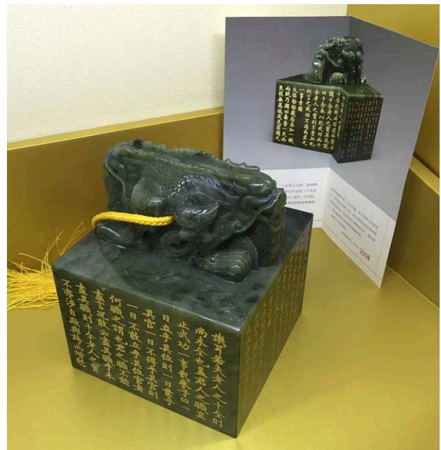
Figure 25. This piece of Manas gray-green nephrite is a 1:1 replica of the imperial jade seal with calligraphy engraving in Qianlong's reign (1736–1795). It was processed by 3D scanning and auto carving. Photo by Mingying Wang.
