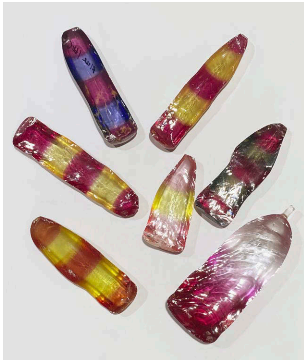
Figure 50. Split boules of bicolor synthetic sapphire grown by flame fusion. Photo by Jennifer Stone-Sundberg; courtesy of RusGems.
