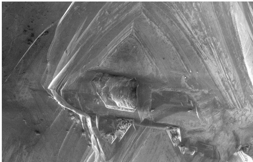
Figure 7. An open channel about 200 \mu\text{m} in width connected the internal cavity with the outside.
