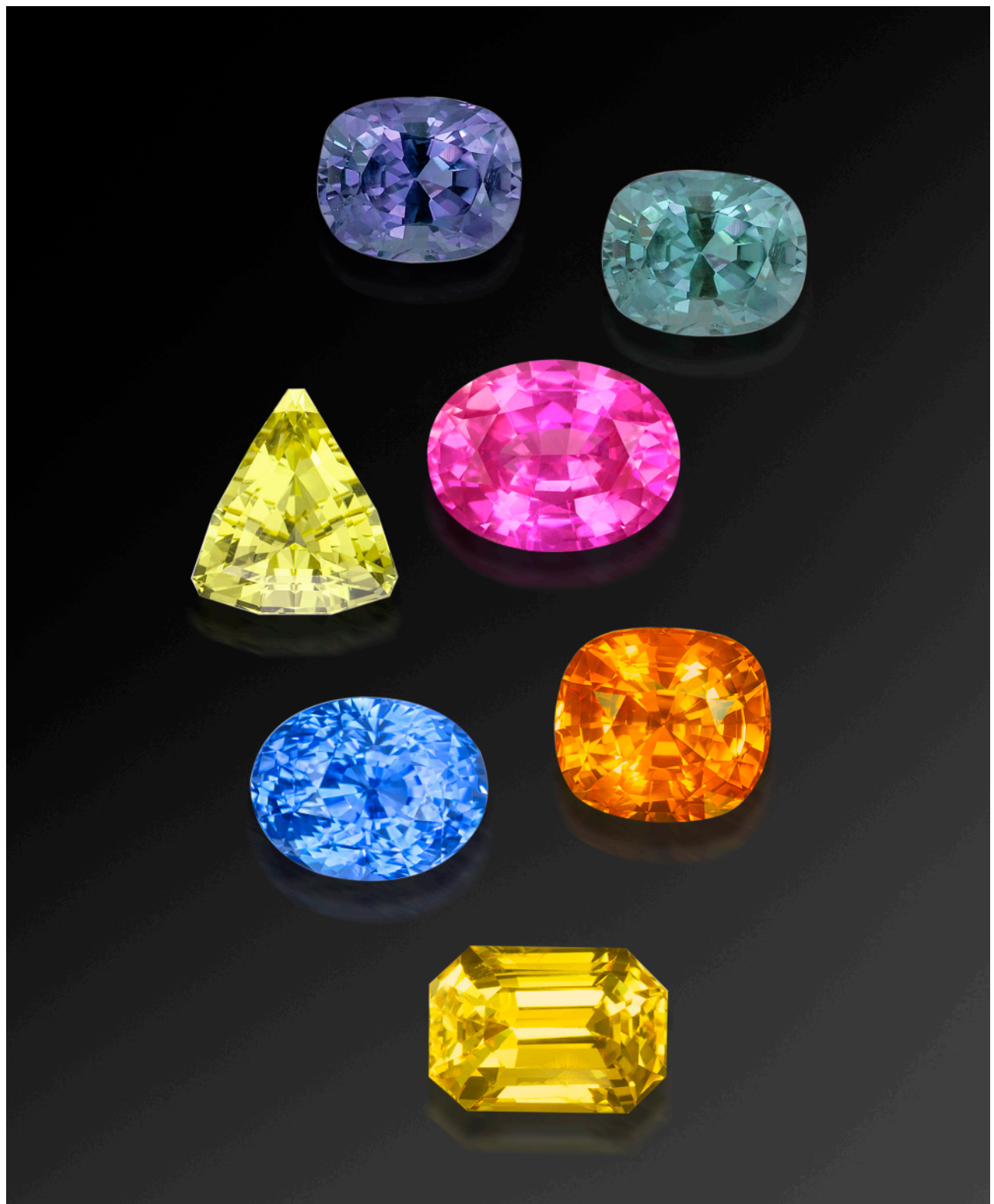
Figure 1. Gem corundum is rarely colored only by a single chromophore; the vast majority are colored by a combination of two or three chromophores. This composite photo illustrates the colors of single chromophores as they would appear in a faceted stone. We searched through a few thousand photos, courtesy of Lotus Gemology, to find these few that closely matched the single-chromophore color circles in this article. These gems represent (clockwise from top left) V^{3+} (first two stones), Cr^{3+} , h^{\bullet}-Cr^{3+} , h^{\bullet}-Fe^{3+} , Fe^{2+}-Ti^{4+} , and Fe^{3+} . Photos by Lotus Gemology.
