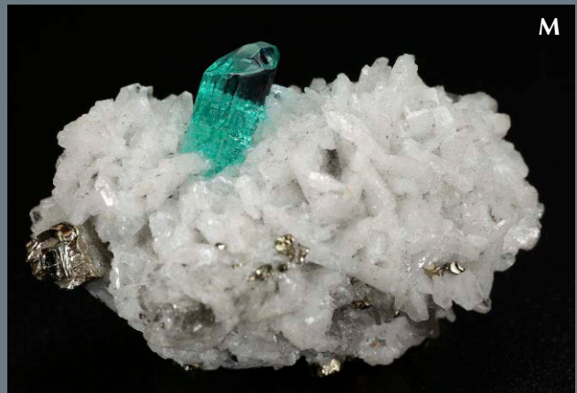
Specimen with emerald crystal Crystal: length 6 mm Habit: hexagonal prism faces terminated by flat basal pinacoids and hexagonal dipyramids Associated minerals: white albite
