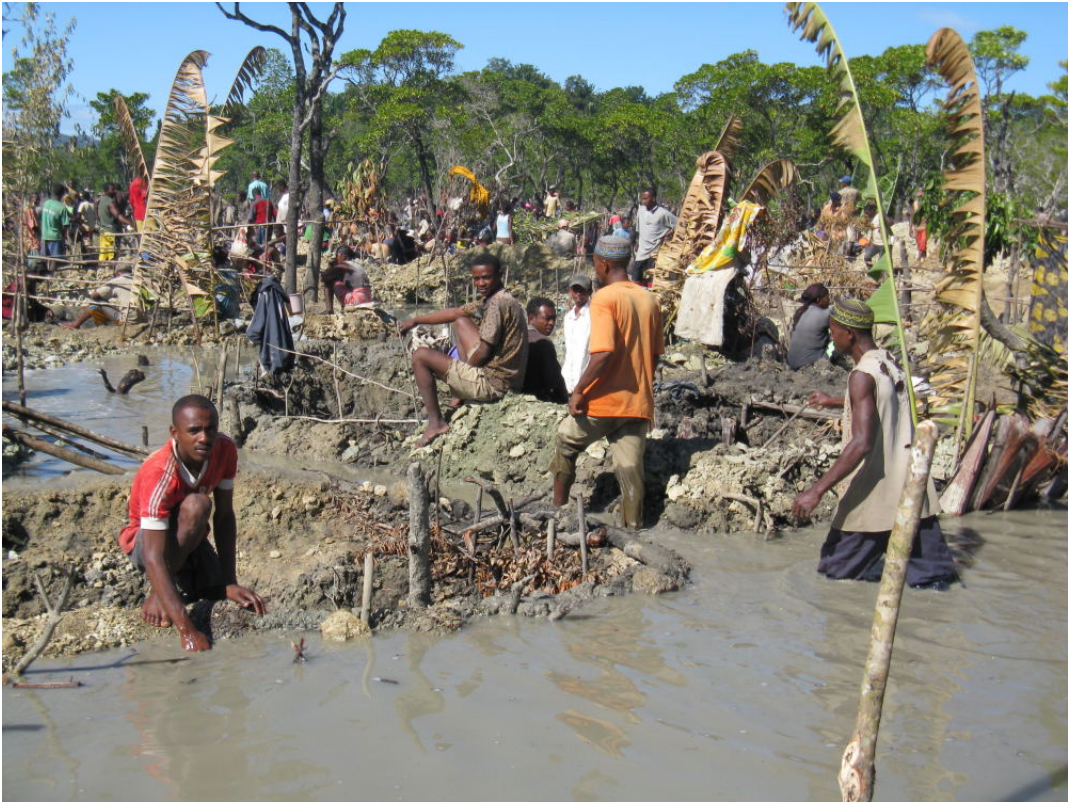
Figure 16. Water is routed away from the pits using a series of canals.
