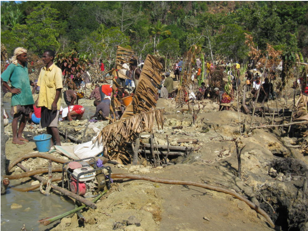
Figure 17. Some miners used gasoline-powered pumps to remove water from the pits.
