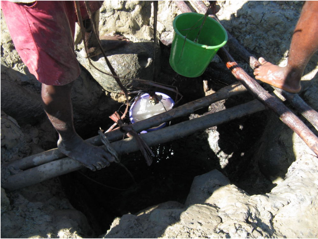
Figure 10. Water is removed from a flooded pit, early in the morning.
