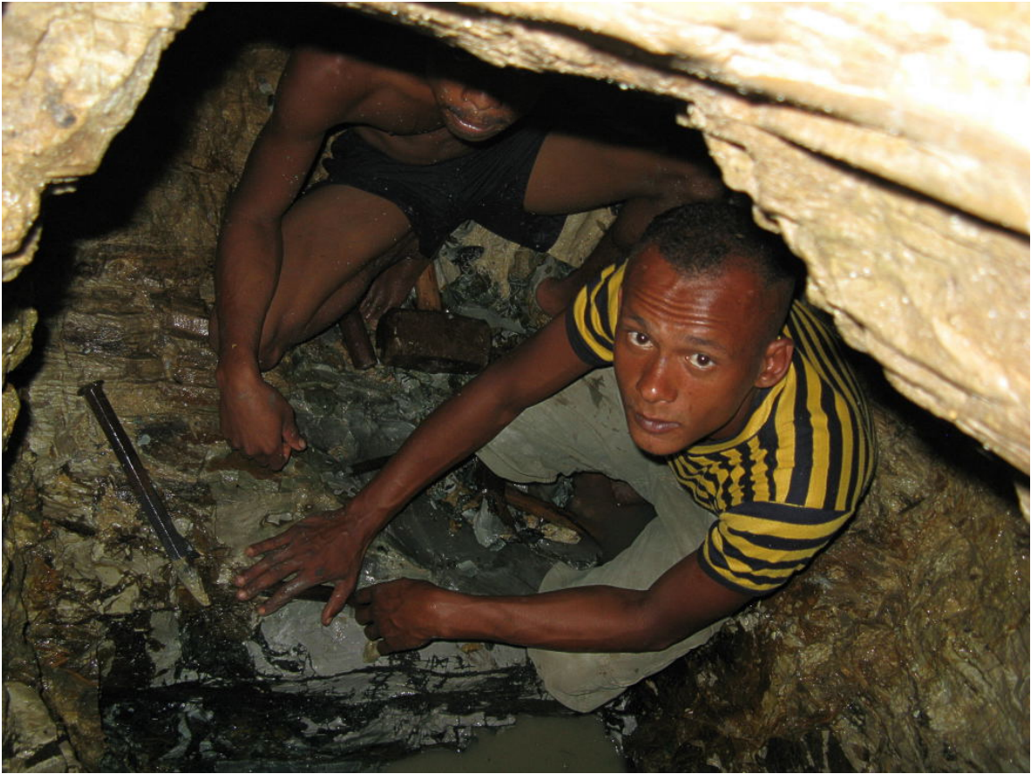
Figure 28. Hammers and chisels are used to penetrate the hard skarn rock.
