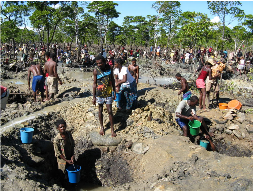
Figure 15. Plastic buckets are used to remove water and mined material from the pits.
