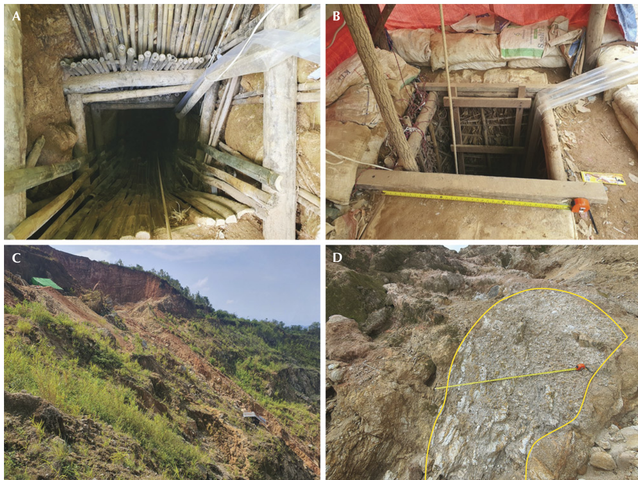
Figure 4. A: Horizontal shafts that gently slope down through the intruded pegmatitic syenite body at Baw Mar. B: Vertical shafts through the overburden biotite gneiss body to the sapphire-bearing syenitic pegmatite. Both shafts measure 1.5 \times 1.5 m. C: A recent view of mining areas at Baw Mar shows small-scale shafts covered with tents. D: Contact between host biotite garnet gneiss and intruded syenitic pegmatite (outlined). The tape measure shown is extended to 1.5 m. Photos by Arkar Moe Myint.
