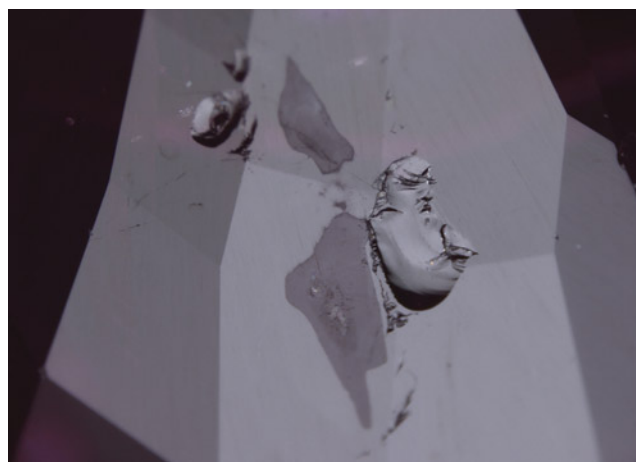
Figure 14. By manipulating different light sources, the filler material is uncovered. While standard lighting shows dull, low-luster patches in the filled cavities (left), fiber-optic illumination reveals a whitish granular texture (right). Photomicrographs by Tsz Wing Lai; fields of view 4.00 mm (left) and 1.50 mm (right).
